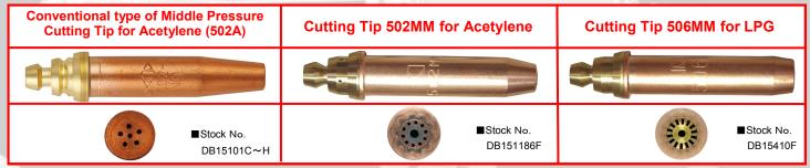
GOLD-MM L/S Cutting Torch & Cutting Tip 500MM have "Tip mixing method" as middle pressure type that preheat oxygen and fuel gas are mixed in cutting tip, so outstanding safety in anti-flash back is greatest feature compared with "Torch mixing method" for low pressure type.
