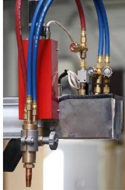
PNC-12 EXTREME oxy-fuel cutting torch package is equipped with high-quality KOIKE cutting torch and automatic on/off solenoid valves on all gas lines, which enables presetting of the flame and automatic piercing sequence. Also, KOIKE 100 series cutting nozzles are included in the package.
