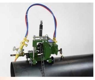
Optional guide rail provides high cutting accuracy, particularly suitable for large pipes.
